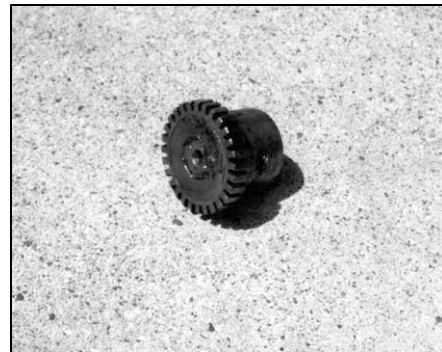
Coupling hub repaired with Loctite Quick Metal.
